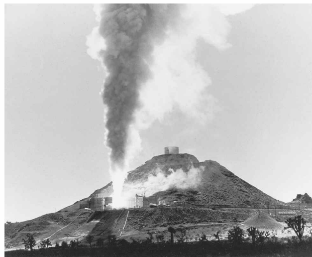
Fig. 8 Extended Length Super HIPPO test at AFRPL. This reusable Nozzle/TVC test system was designed to emulate Stage 1 Peacekeeper pressure, throat size, and duration. In the largest configuration, the 2-m diam, ~10-m long motor burned 40,000 kg of propellant at 9.7 MPa (1400 psi) for 58 s to test nozzles with throats almost 0.4 m in diam.
