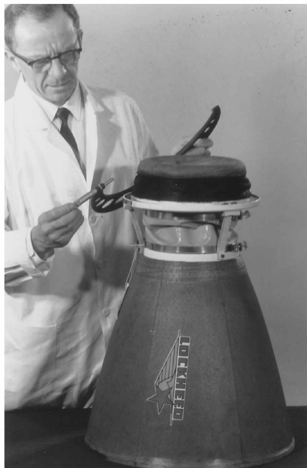
Fig. 6 Solid rocket thrust vector control became more robust via a series of extraordinary inventions. The Lockseal nozzle, shown with John Herbert (one of its inventors), has proven best for most TVC systems since its debut in the 1960s.
