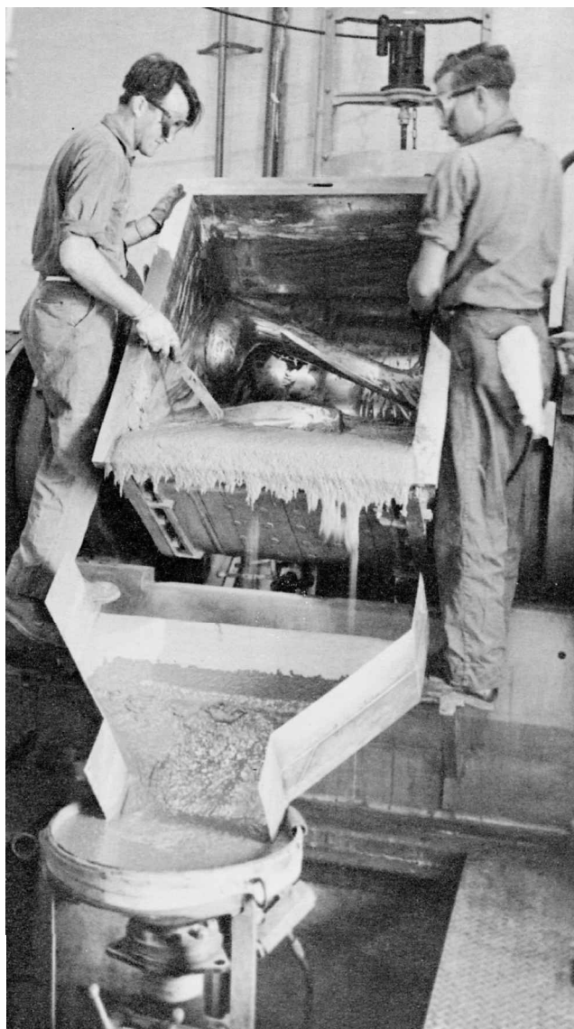
Fig. 1 Mixing propellant was a hands-on operation in 1957. Crew is discharging a 100-gallon Baker-Perkins mixer at Thiokol Elkton. The propellant is polysulfide and ammonium perchlorate.
